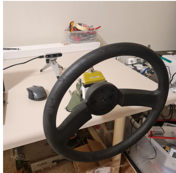
Figure 4. Complete setup for capturing steering gestures.
