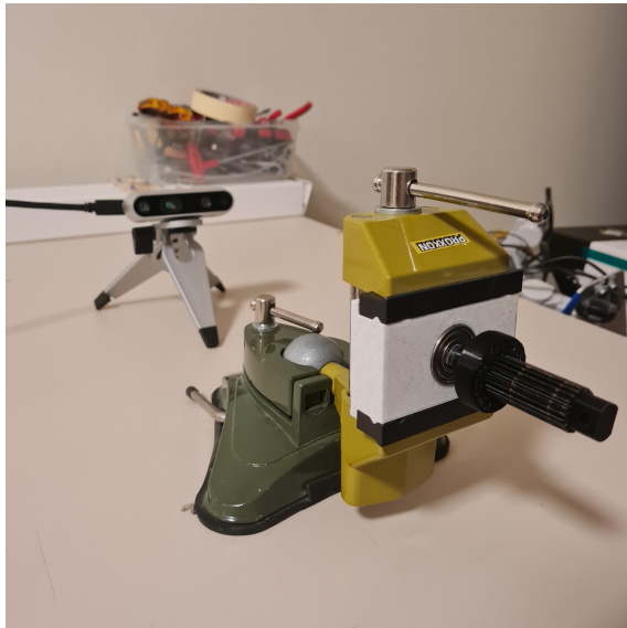
Figure 3. 3D-printed mount for stable steering wheel positioning.
